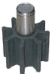
Liverani's flexible impeller pumps are made of food grade rubber that rotates inside an eccentric Stainless steel housing. Flexible impeller pumps are simple and economical to use, they are self priming and capable of lifting wine up to six meters. Due to the forgiving nature of the rubber impeller, they can pump liquids with suspended particles such as seeds and skins without damage.
