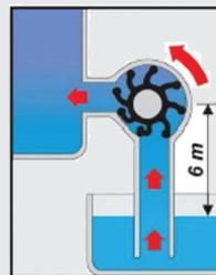
Self-priming (automatic priming of the product up to 6 meters even from dry start-up.
